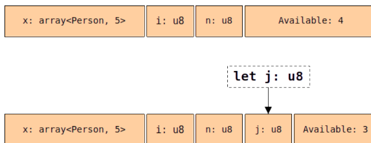
Figure 10.1: Available slots are split when a smaller variable is allocated to them.
